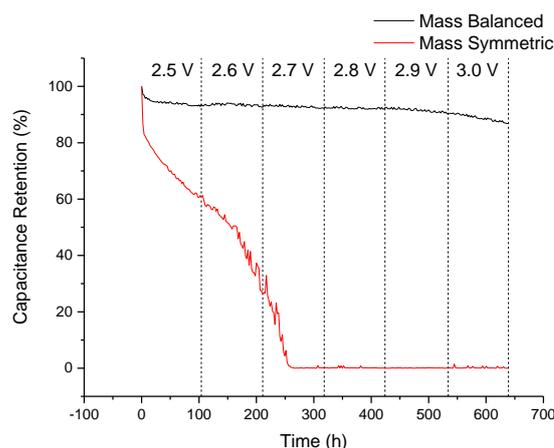
**Figure 2:** Cell capacitance retention with respect to time during cycling for mass symmetric ( $m^+/m^- = 1$ ) and mass balanced ( $m^+/m^- = 2.4$ ) cells up to different sequential cut off voltage ranging from 2.5 to 3 V for 1 M TEABF<sub>4</sub> in ACN.
