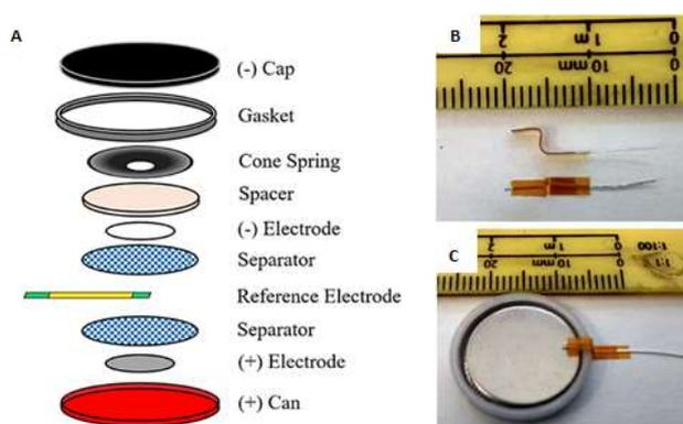
**Figure 1:** **A)** Schematic showing the setup of incorporating the Ag wire QRE within the CR2032 coin cell. **B)** and **C)** Images showing the Ag wire QRE and its incorporation.
