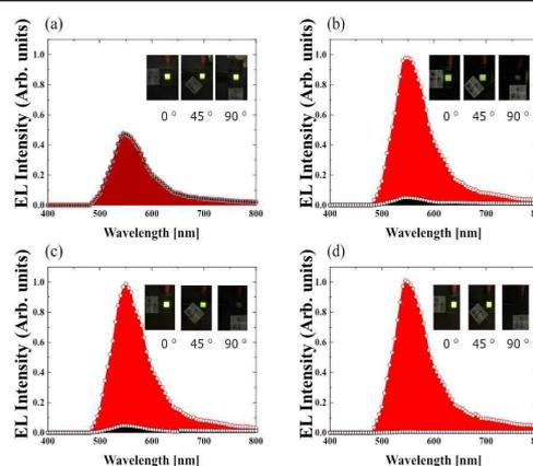
**Figure 1:** EL spectra of (a) N-MoS<sub>2</sub>-, (b) R-MoS<sub>2</sub>-, (c) I-MoS<sub>2</sub>-, and (d) RI-MoS<sub>2</sub>-based OLEDs. The output spectra taken when the transmission axis of the polarizer was 0° and 90° are shown in red and black, respectively. The insets are optical images of OLED devices obtained at different rotation angles (0°, 45°, and 90°) of the polarizer.
