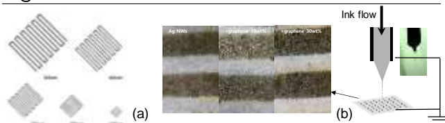
Figure 1: (a) Screen-printed graphene paste circuit lines on colorless polyimide (100 to 500 μm) (b) Line patterns of graphene and graphene/silver nanowire composites on paper by EHD jet-printing
