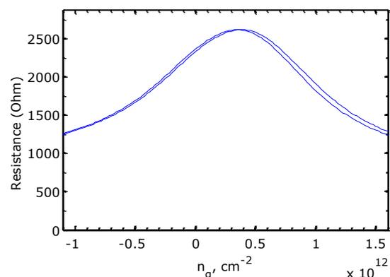
**Figure 1:** Graphene device on SiO<sub>2</sub>, fabricated using thin Cu-film catalyst on single crystalline sapphire showing low hysteresis and low doping.
