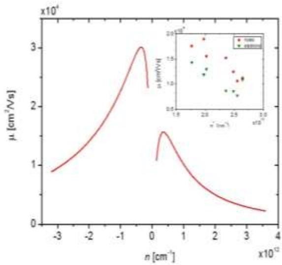
**Figure 2:** Room temperature field effect mobility of wet transferred CVD graphene encapsulated between hBN flakes and with thermal post-treatment. The inset shows correlation between mobility and residual doping  $n^*$  for CVD graphene on hBN for various samples
