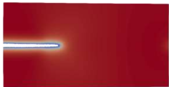
Figure 2: Crack propagation obtained from a phase-field simulation assuming a homogeneous material.
