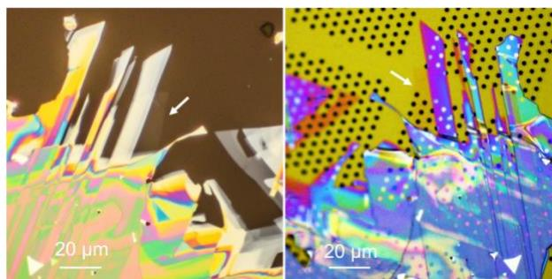
**Figure 1:** Optical micrographs of the GaSeTe sample exfoliated onto PDMS (left) and directly transferred onto a SiN TEM grid (right). The white arrows show the location of the ultrathin GaSeTe crystal on PDMS and TEM grid.
