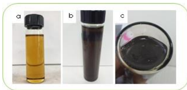
Figure 1: a) neat lubricant; b) well dispersed functionalized GO in lubricant; c) excellent dispersion with clear bottom of vial without apparent sedimentation of functionalized GO.
