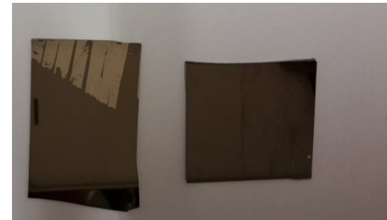
Poor adhesion of metal contacts to graphene.
