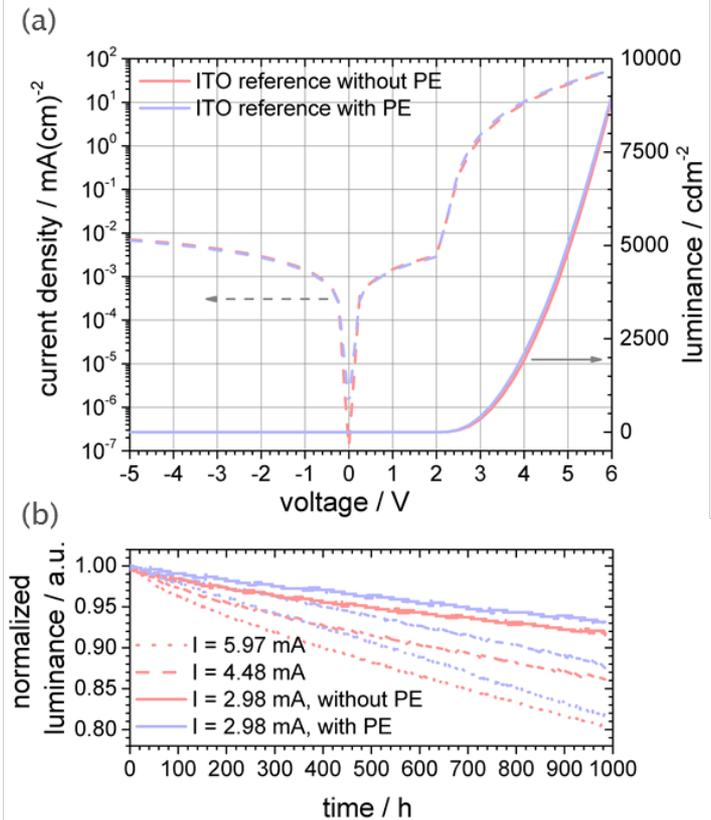
Figure 3. (a) Luminance–current density–voltage (LJV) curves of ITO reference samples containing a hole transport layer which has not experienced any plasma etching (light red) and which has (light blue) as well as the corresponding luminance decay curves determined at three different currents.
