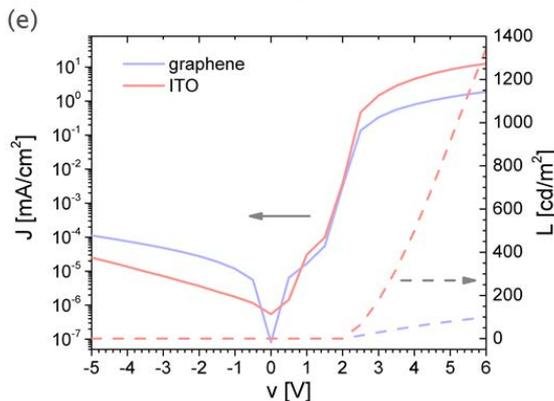
Figure 5. Example of a flexible, transparent OLED with an emitting area of 1.5×2 (cm)<sup>2</sup> after patterning it by plasma etching (a–d) and its JV characteristic compared to the ITO reference.
