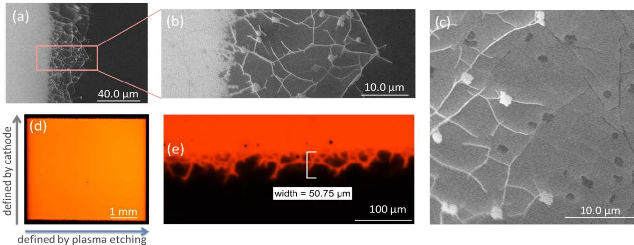
Figure 4. (a) and (b) present SEM images after the plasma has been applied for 120 s resulting in an HTL reduction of 5.1 nm: on the left side a 15 nm thick, amorphous HTL layer (light grey) is seen with a 40 – 50 μm wide transition zone. (c) detailed image of (b) indicating the presence of graphene islands and boundaries. (d) and (e) present microscopy images of resulting OLED devices demonstrating that this transition zone has a width of the same magnitude.
