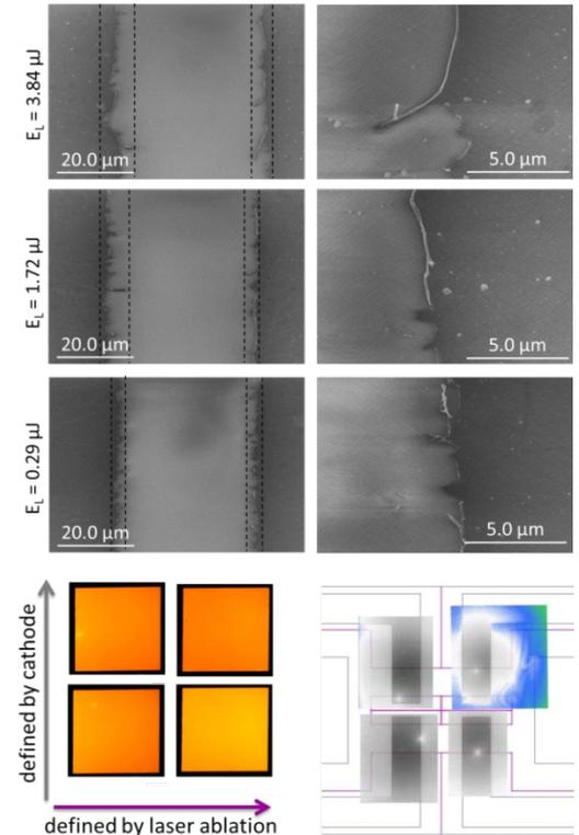
Figure 2. (Top, right) SEM pictures of graphene edges on glass after laser ablation in dependence on the radiant fluence, (bottom, right) as well as corresponding thermographic images of resulting OLED devices. (Left) 2D Raman map of separated graphene layers by laser ablation.
