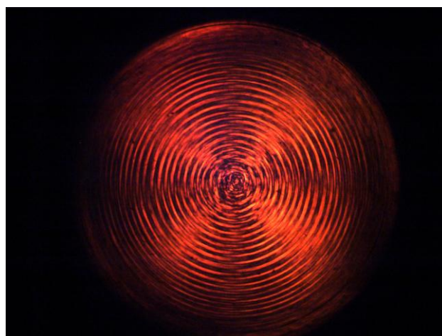
Figure 1: SIPLI image of GO suspension sheared in plate-plate geometry (shear rate at the sample edge is 100 rad/s). The Maltese cross indicates overall alignment along the flow, whilst the banding results from helical vortices.
