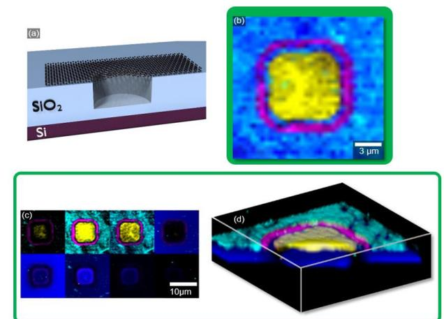
**Figure 2:** a) cross-section schematic of one device; b) 2D-Raman scan of one cavity from the test structures (top view) indicated by a green square in Fig. 1c; c) Sequence images of a cavity for the taken at different z-positions; d) 3D tomography image of a cavity.
