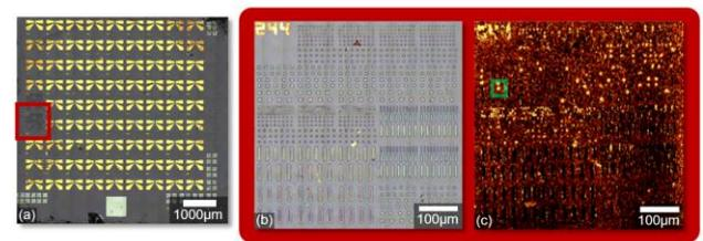
**Figure 1:** a) Stitched white light image of the complete chip; b) stitched white light image of the test structures; c) Raman image of the test structures displaying 2D peak intensity (yellow: intact membrane; black: broken membrane).
