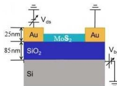
**Figure 1:** Schematic “cross-sectional” view of the device
