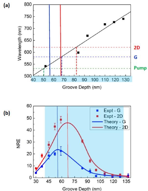
**Figure 2:** (a) Maximized total absorption wavelength variation with groove depth. (b) Normalized Raman enhancement variation with groove depth for G- and 2D-peaks. Dots represent experimental data points and solid curves are theoretical fits (EM simulations).
