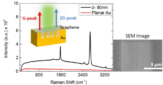
**Figure 1:** Raman spectrum of graphene on planar Au (red curve), graphene on groove-arrays with a width of 75nm and depth of 80nm (black curve). SEM image of the fabricated gratings. Inset: SERS platform schematic
