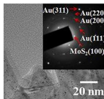
**Figure 1:** Au-MoS<sub>2</sub> with inset showing selective area electron diffraction pattern.
