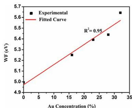
**Figure 2:** Variation of work function of Au-MoS<sub>2</sub> with respect to Au concentration.
