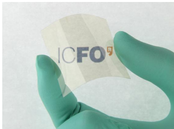
Figure 1: Flexible PEN coated with graphene and a QD thin film (20nm) is highly visibly transparent and photosensitive. These sensors can be integrated into wearables, flexible displays, and more.
