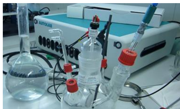
Figure 2: Three-electrode cell for CDI tests.
