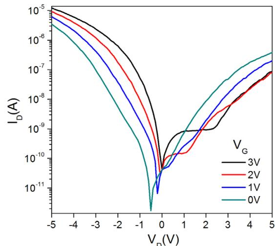
Figure 2:  $I_D$ - $V_D$  electrical characteristics as a function of gate bias
