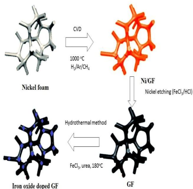
**Figure 1:** Schematic illustration of synthesis of iron oxide doped graphene foam
