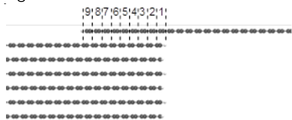
Figure 1: Structure of the graphene on graphite contact with a varying finite amount of overlap.
