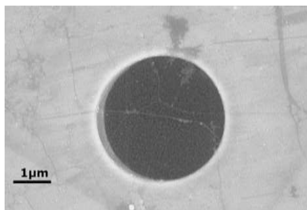
Figure 1: SEM image of graphene drum resonator with diameter \sim 5\mu m.
