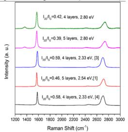
Figure 2: Normalized Raman spectra of fewlayer graphene (FLG) particles from different sources. Green and magenta spectra were obtained during the present work, while blue [3], red [1] and black [4] spectra are from literature for 4- and 5-layer graphene particles.
