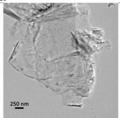
**Figure 1:** Transmission electron microscopy bright-field image of a Graphenest sample.
