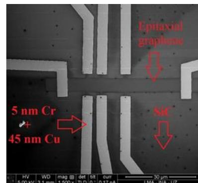
**Figure 2:** SEM imaging after lithography to establish metal contacts to epitaxial graphene grown on SiC substrate
