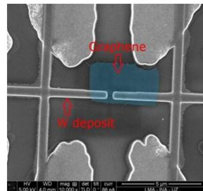
**Figure 1:** SEM imaging of CVD-graphene on top of metal contacts
