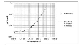
Figure 1. Inverse of the mobility vs. defect concentration.
