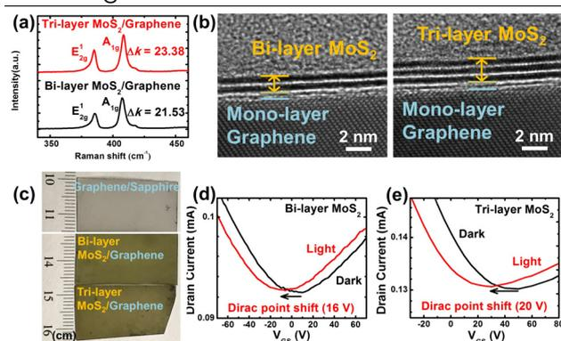
**Figure 2:** (a) The Raman spectra, (b) the cross-sectional HRTEM images and (c) the pictures of the bi-layer and tri-layer MoS<sub>2</sub>/graphene samples. The I<sub>D</sub>-V<sub>GS</sub> curves of the (d) bi-layer and (e) tri-layer MoS<sub>2</sub>/graphene phototransistor under dark and light irradiated conditions at V<sub>DS</sub> = 1V.
