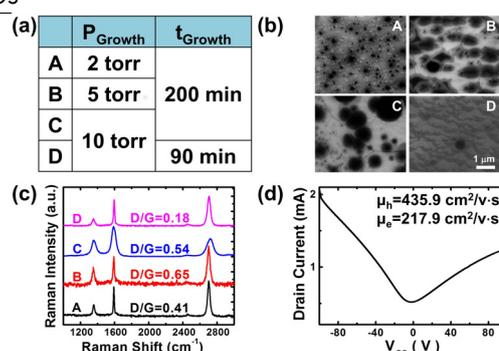
**Figure 1:** (a) The growth parameters, (b) SEM images and (c) Raman spectra of the four samples. (d) The I<sub>D</sub>-V<sub>GS</sub> curve of the graphene bottom-gate transistor at V<sub>DS</sub> = 1 V.
