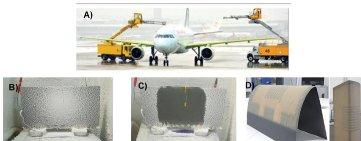
Fig. A: Typical de-icing process of an airplane through propylene glycol spray.
