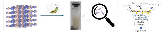
**Figure 1:** Schemes of h-BN exfoliation from raw powder up to h-BN stabilized in solution (left) and screening method to select the best h-BN/surfactant combination (right).
