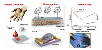
Figure 1: A schematic illustration of the concept of the cytokine sensor operation.
