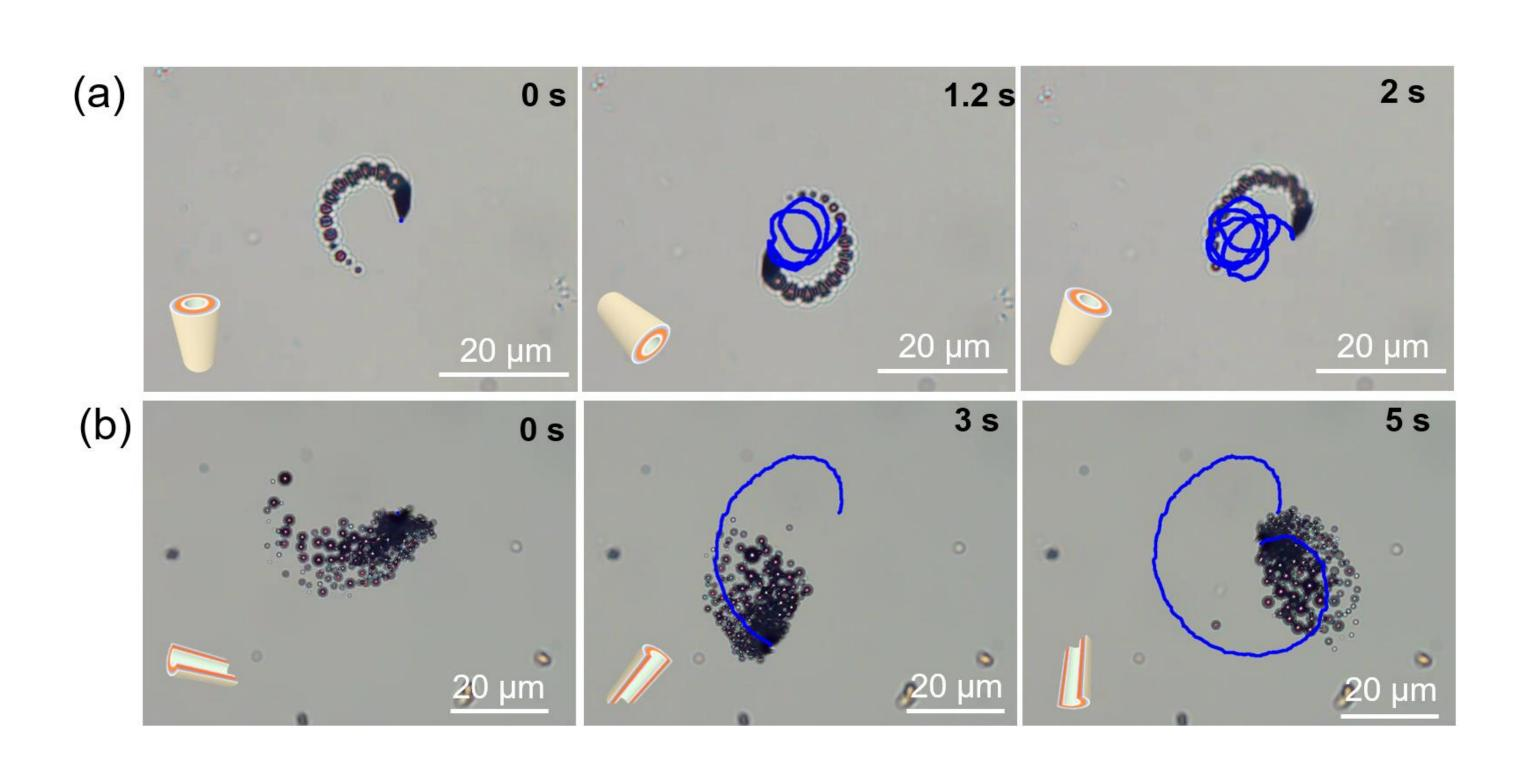
Time-lapse microscope images of (a) a tubular micromotor and (b) an arc micromotor moving in 5% H<sub>2</sub>O<sub>2</sub> and 0.125 wt% SDS. The tracked trajectories of micromotors were highlighted in blue.
