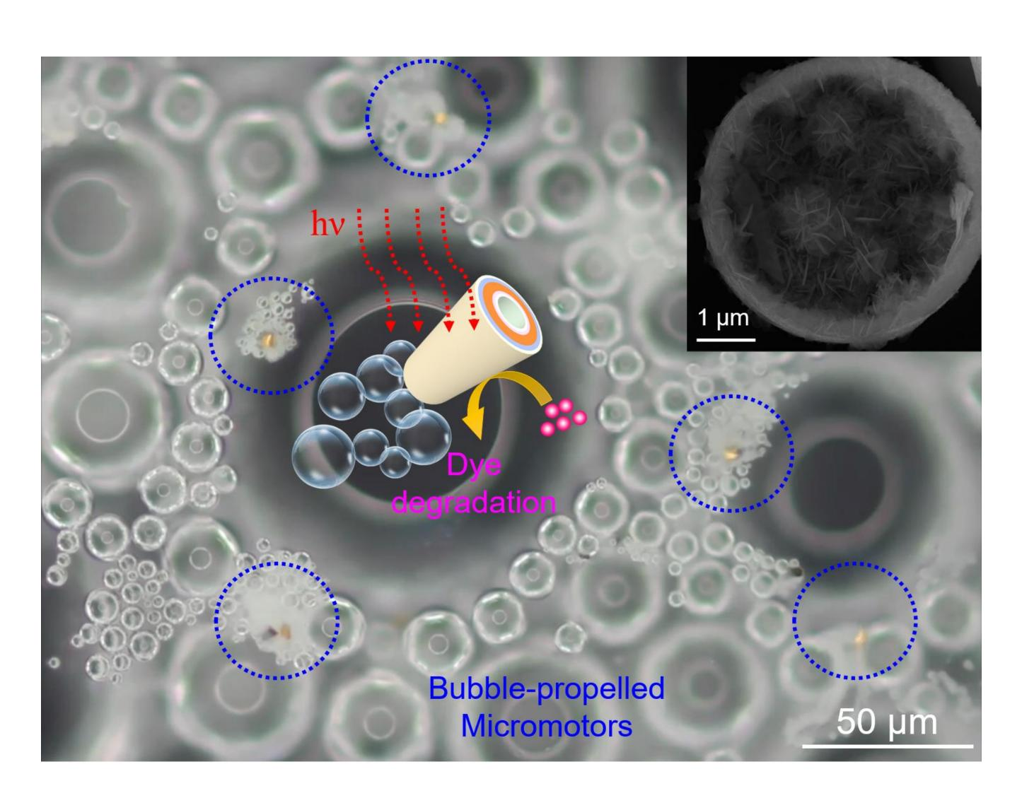
Collective behavior of bubble-propelled BiOI-based micromotors for the photocatalytic degradation of pollutants in the contaminated water under the illumination of visible light. The micromotors were highlighted via blue dashed cycles.
