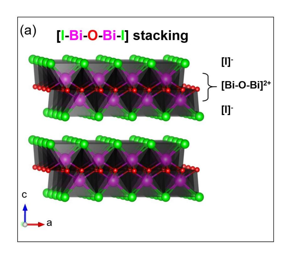
Layered crystal structure of BiOI with stacked [I-Bi-O-Bi-I] drawn by VESTA software.
