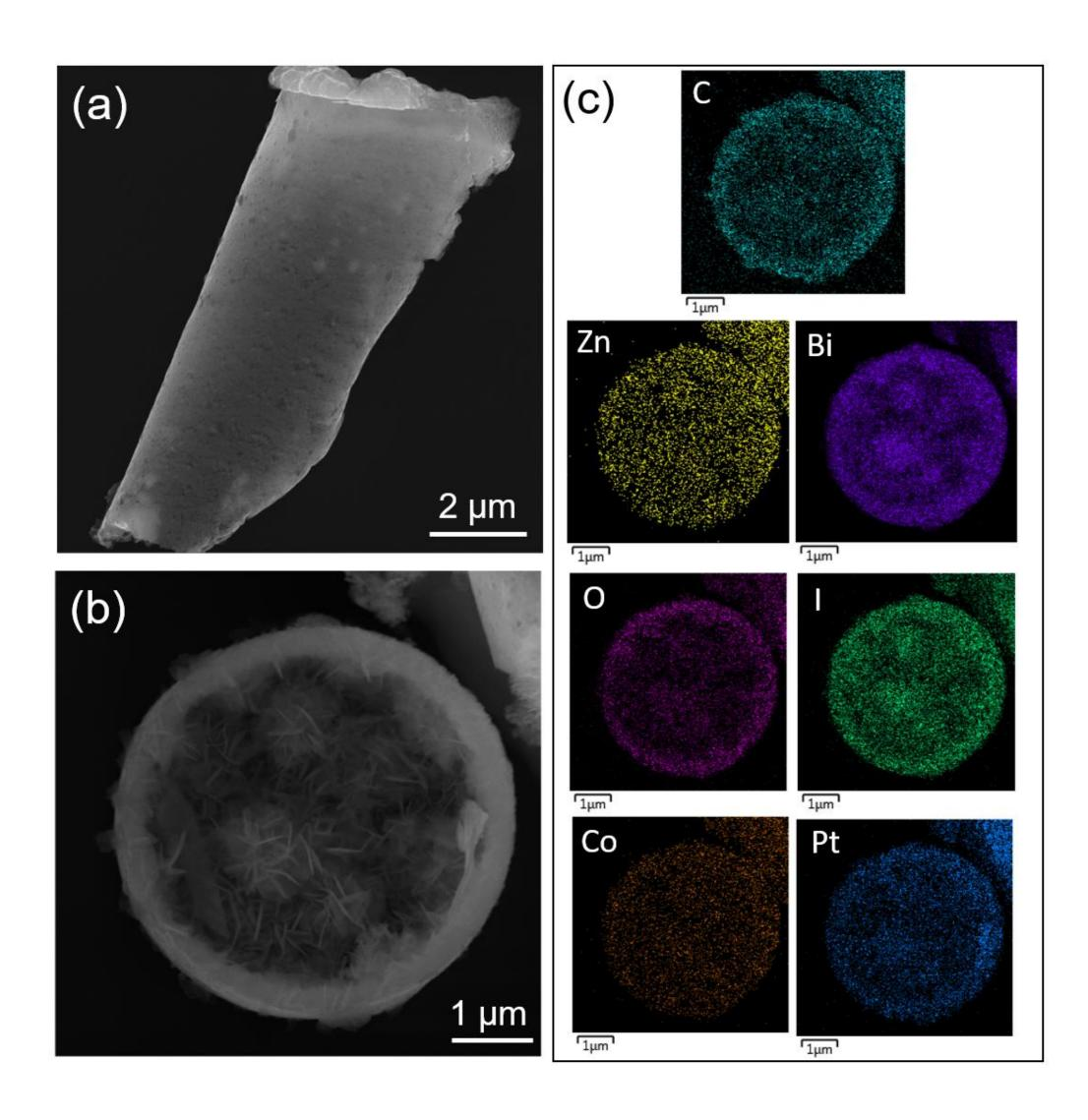
(a) SEM image of BiOI-based micromotors. (b) Cross-sectional image of micromotors and corresponding (c) elemental composition from EDX analysis.
