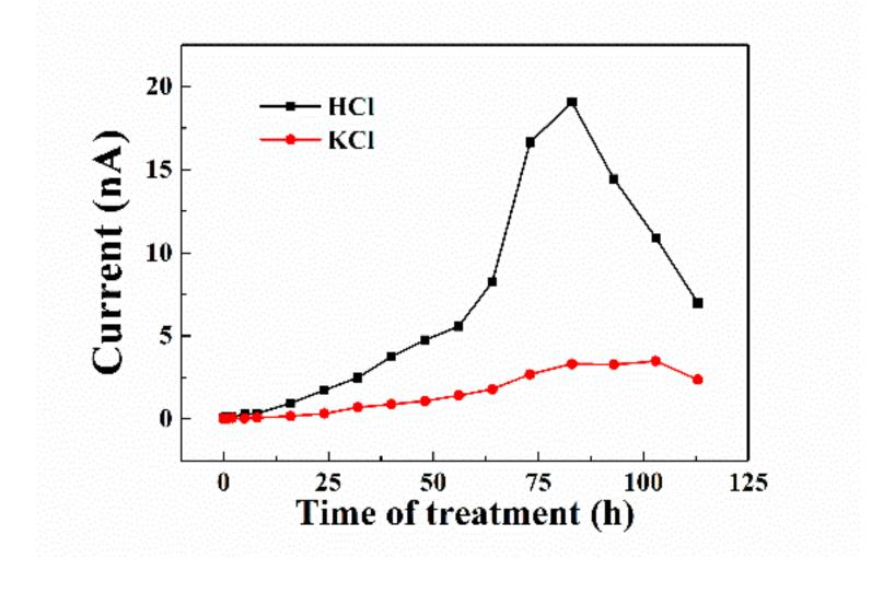
Ionic current measurements tracked the conductance variation with treatment time in 0.1 M solutions.
