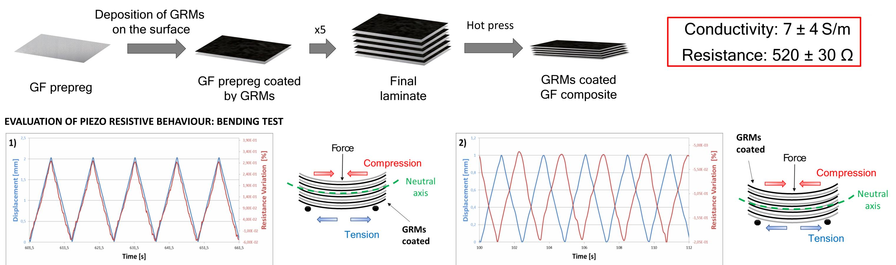
The samples show two different piezo resistive behavior depending on the samples side:
