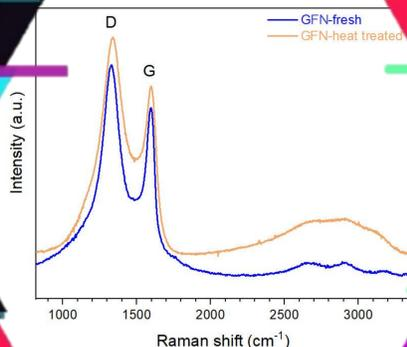
Figure 5. Raman spectra of GFN material before and after heat treatment (at  $1000 \text{ }^\circ\text{C}$  in an argon atmosphere).
