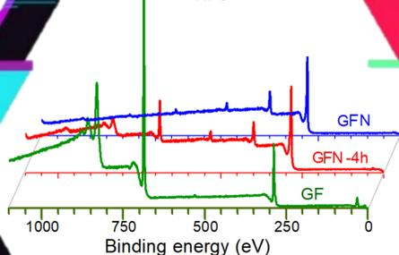
Figure 1. XPS survey spectra of starting material (GF), byproduct (GFN-4h) and final GFN material. The final material had 16 at% of N.
