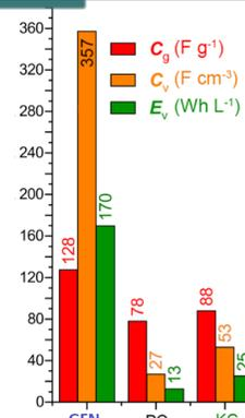
Figure 6. Comparison of the GFN cell with symmetric cells made using commercial high surface area porous carbons (PC and KC) at  $2 \text{ A g}^{-1}$ .
