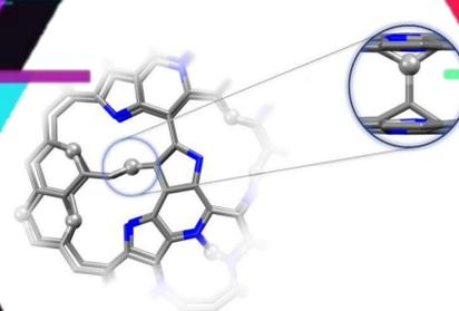
Figure 2. Theoretical model of GFN structural fragment (C:N atomic ratio of ca. 84:16) optimized by DFT calculations. The formed interlayer bonds are highlighted as spheres. The model simulates the structure only locally (few-atom level).
