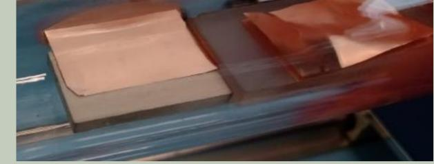
During our experiments of graphene growth at elevated temperatures a problem we encountered was that part of the copper would get stuck to the quartz boat, causing wrinkling of the copper during cooling. We solved this by substituting the quartz boat with a BN boat, to which the copper will not get stuck due to the low metal wettability of BN.
