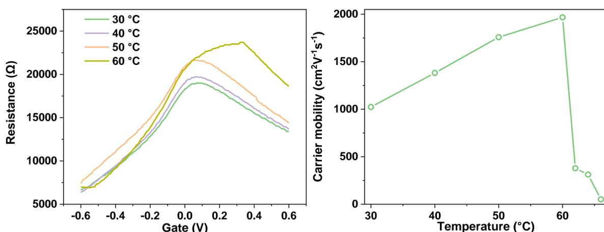
The transfer curve of GFET/PCL moved slowly upward as the temperature gradually raised. When it started to reach the melting point at 60 °C, the transfer curve showed a big change. Its carrier mobility increased as well. We know that temperature has little effect on the carrier mobility of graphene, so it can be inferred that the PCL polymer substrate releases the stress in graphene and improve its carrier mobility when it changes from solid to liquid<sup>[2]</sup>.
