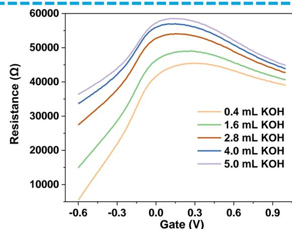
The pH sensing response was measured at 60 °C. The transfer curve changes regularly as the content of KOH increases, demonstrating that GFET/PCL can detect the amount of KOH and the pH as well.
