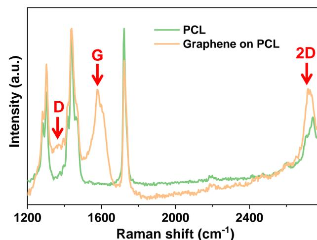
By comparing the Raman spectra of PCL and graphene on PCL, the good quality of graphene can be revealed.
