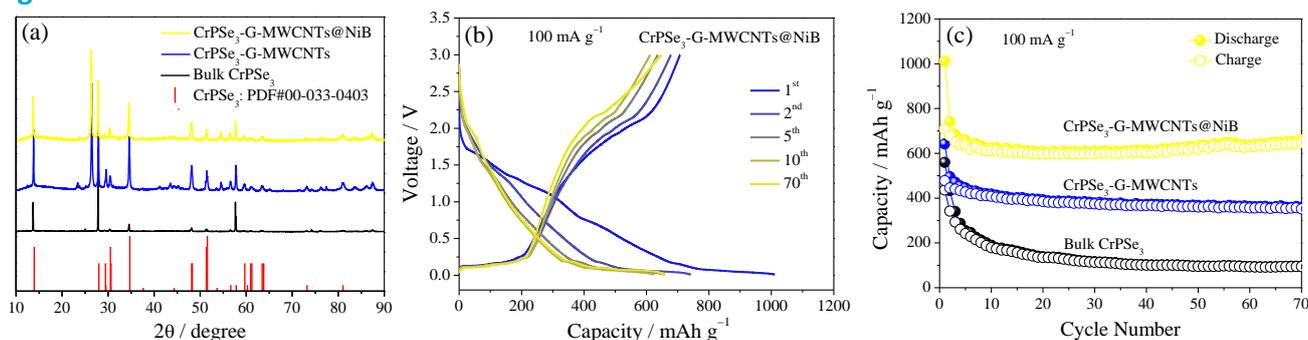
**Figure 1:** (a) XRD patterns of bulk CrPSe<sub>3</sub>, CrPSe<sub>3</sub>-G-MWCNTs, and CrPSe<sub>3</sub>-G-MWCNTs@NiB composites; Cycling response of (b, c) bulk CrPSe<sub>3</sub>, CrPSe<sub>3</sub>-G-MWCNTs, and CrPSe<sub>3</sub>-G-MWCNTs@NiB in two-electrode half-cell at 100 mA g<sup>-1</sup> current density in terms of (b) voltage profiles of selected cycles and (c) cycling trend.
