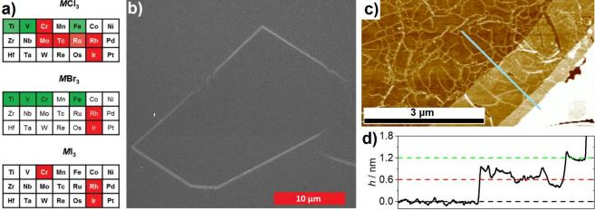
**Figure 1:** a) overview of transition metal trihalides with 2D structure (red: AlCl<sub>3</sub>-type, green: Bil<sub>3</sub>-type) [1], b) SEM image of an as grown Cr<sub>x</sub>Ru<sub>1-x</sub>Cl<sub>3</sub> nanocrystal with a height of ca. 30 nm (surface particles and cracks can be attributed to carbon sputtering), c) AFM image of a Cr<sub>x</sub>Ru<sub>1-x</sub>Cl<sub>3</sub> fewlayer structure obtained by delamination, d) height profile of the in c) shown step of a mono- and bilayer.
