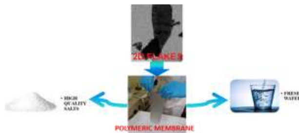
Figure 1: Inclusion of 2D flakes in PVDF-based membrane for desalting highly saline waters and recovery salt crystals [3]
