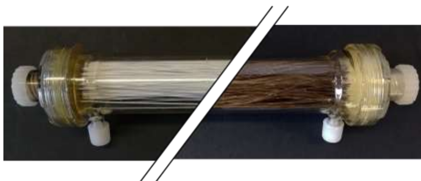
Figure 1. A hollow fiber microfiltration module before (left) and after (right) functionalisation with GO.
