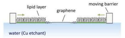
Graphene (pristine or chemically functionalized) floating on the surface of water is subject to the external compression from a lipid layer in a Langmuir-Blodgett trough
