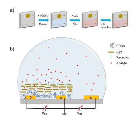
Figure 1: Schematics of the preparation of the test pattern (a), DC operation of the rGO-LGT (b).
