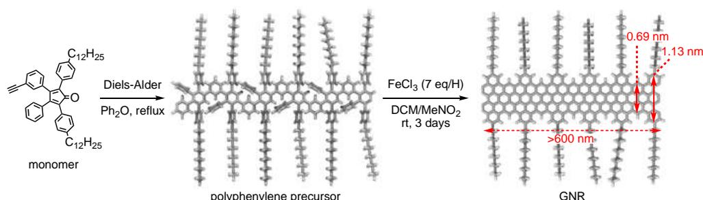
Figure 1: An example for bottom-up solution synthesis of graphene nanoribbons.<sup>[3]</sup>
